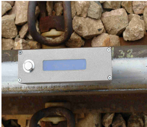
Fig. 2. Electronic level during the field tests
