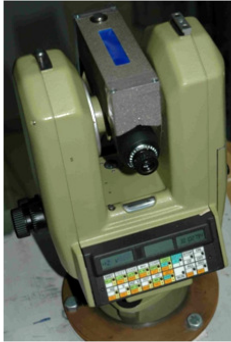
Fig. 3. Electronic level with electronic total station Leica TC2002 during testing in geodetic metrology laboratory of AGH University of Science and Technology
